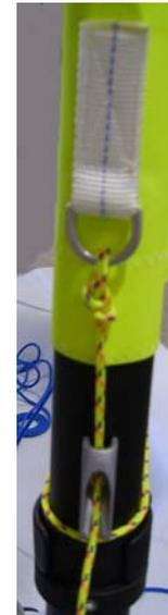
6. Tie a **stopper knot** in the end of the **outhaul**, and thread it through the right-hand hole at the end of the **boom**, around the outhaul hook, and through the left-hand hole at the end of the **boom**.
