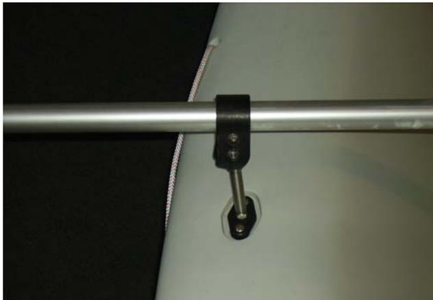
To locate and lock the oars in position, push the spigot in the [rowlock hole](#) (fig 5.8) and rotate the complete oar, so that the paddle is over the [cockpit](#) and the handle is over the side of the boat. As you turn the oar into the correct position, with the paddle over the side and the handle over the [cockpit](#), you will feel the oar lock into place (fig 5.9). The oar will not pull out. To release the oar, reverse the procedure.
