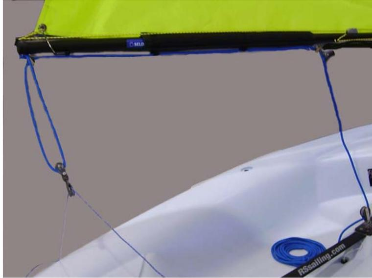
**15.** Thread the **mainsheet** through the **mainsheet centre block**, making sure that it is in the right direction for the ratchet to work. Tie a knot in the **mainsheet** so that the **boom** cannot pass beyond a 90° angle to the **hull centreline** when you are sailing.
