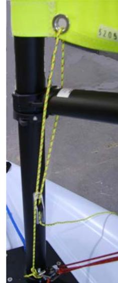
Sport Sail: Tie the **downhaul** on to the metal ring on the sail sleeve, then pass it through the **cleat** on the front of the **mast**. If you also have a Pro sail, coil and tie off the excess **downhaul**. If you only have a Sport sail, you can cut off the excess **downhaul**.
