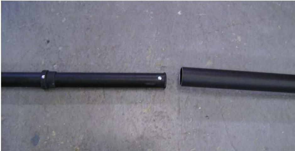
2. Push the mast top section in until it hits the stop.
