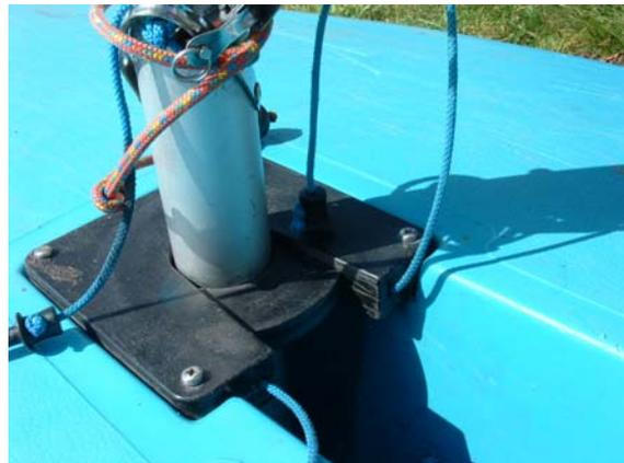
Push the boom onto the mast just above the mast locating collar.
