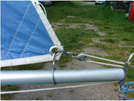
Connect the outhaul to the clew of the sail. Also connect the boom ring to the clew of the sail. The outhaul should be fairly slack unless it is very windy ... in which case pull it tight.
