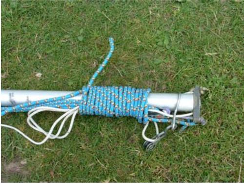
Wrap the end of the mainsheet around the end of the boom and the outhaul. Tuck in the end.
