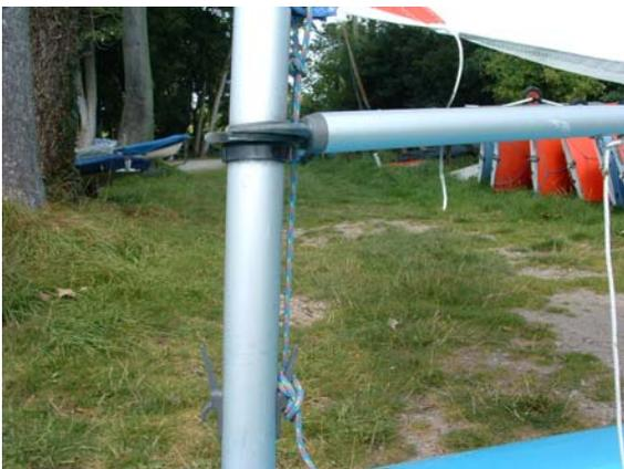
Note the outhaul location (the white rope) should already be fitted as shown here.
