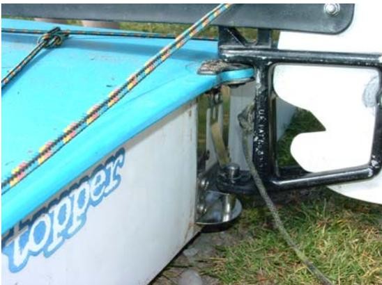
Topper rudders sink (!) so be sure to tie the rudder onto the forward part of the sheet horse. Make sure the tie rope goes under the back part of the sheet horse.
