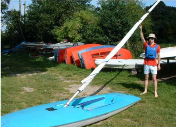
With the mast gate open, insert the mast/sail assembly at this angle. As the mast reaches a vertical position, it should drop down into the mast step with a “thud”.
