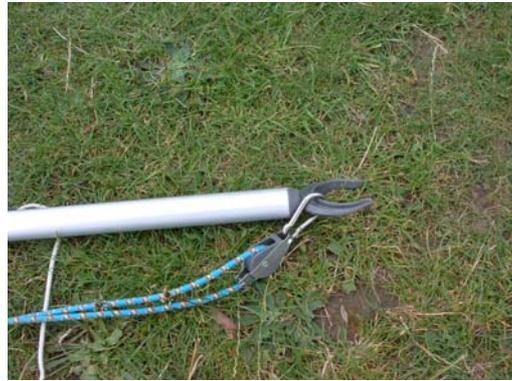
Pulling from the boom front mainsheet block, tighten the mainsheet.
