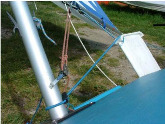
You won't be able to put your dagger board into place until you are on the water ... when there is enough depth of water, slide in your dagger board (the elastic is to the front), pass round the boom and clip back onto the elastic. The elastic should hold the dagger board into the position you choose ... if it is too loose, pass it around the mast again until it does hold the dagger board in place.
