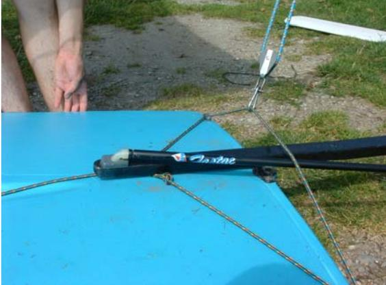
Take the rudder/tiller assembly and from aft, push it under the sheet horse. Pull the tiller extension clear ...
